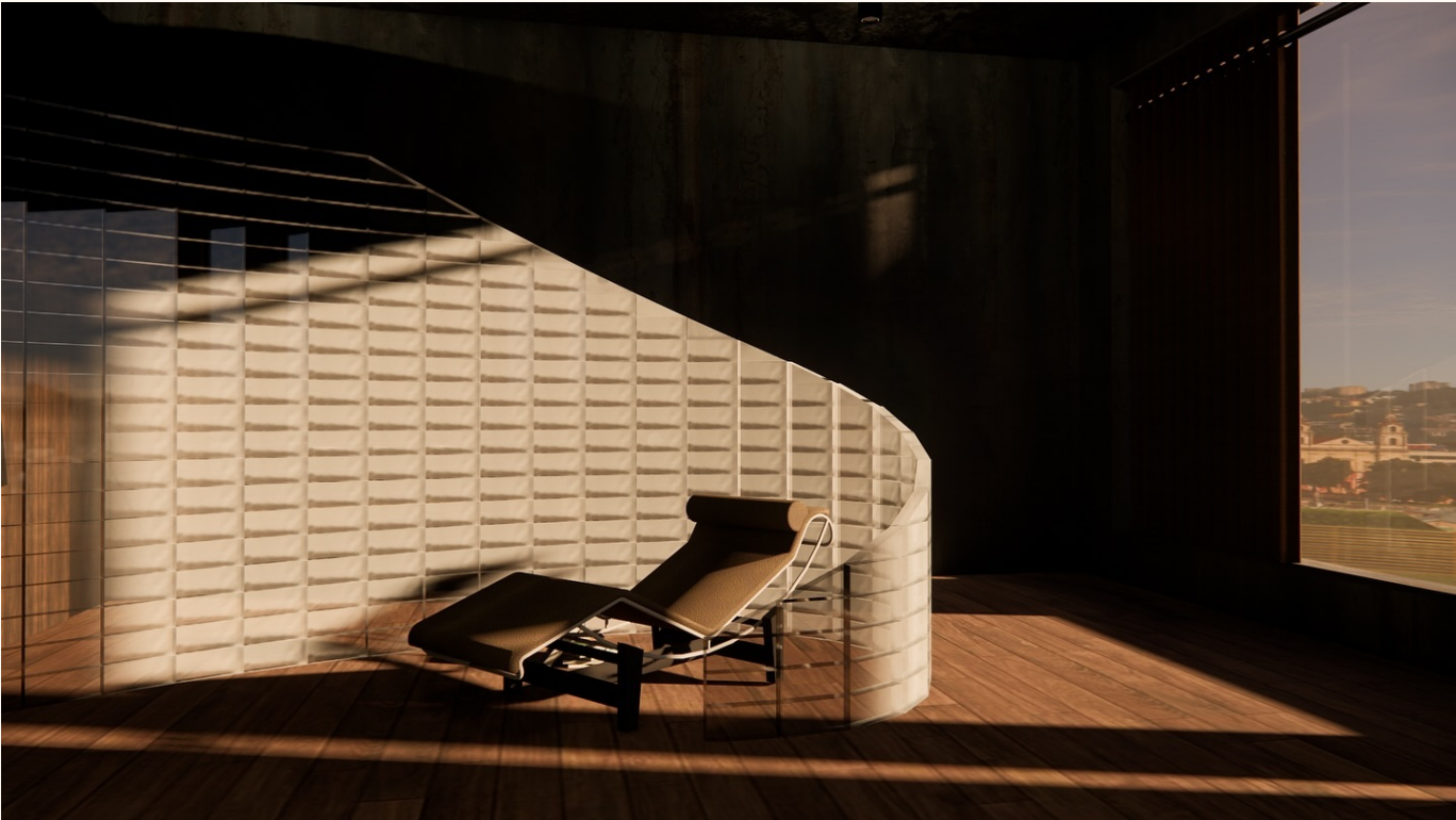
03.1 Lounge. A curved glass block wall draws daylight into the interior.
